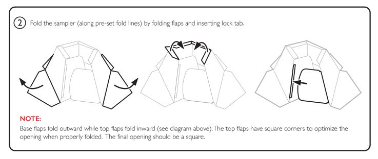
Place the sampler over the threat, wait 1 minute, then measure with AP4C / AP4C<sup>+</sup> up to 30 seconds.
